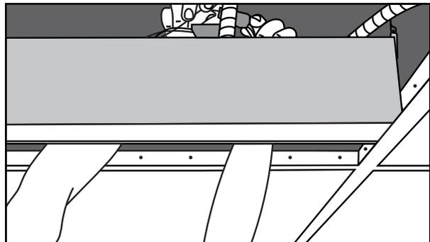
**Step 4:** Connect pigtail disconnects to luminaire disconnects. Insert wires into housing. Insert knockout plate and fasten using screw provided.
