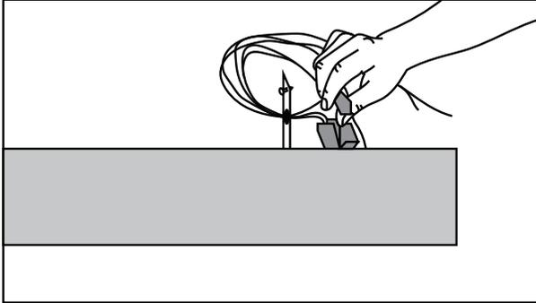
**Step 1:** Shut off power. Remove ceiling tile from desired light fixture location. Remove knockout plate. Remove pigtail.
