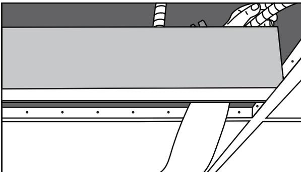
**Step 3:** Lay luminaire in grid at desired position. Secure fixture to structure above using structural wire (by others) via holes in the end plates.
