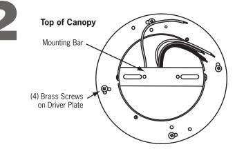
There should not be any excess cable in the ballast compartment. Leave only 6-8" for wiring available.
