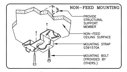
ELECTRICAL BOX (PROVIDED BY OTHERS.) SEE NOTE 1. 8-32 X 7/8" TRUSS HD. **SCREW** 0551200A MOUNTING STRAP-0391570A 5/64"ALLEN WRENCH BALL-0553080A SWIVEL 0391560A 1" X 5-1/4" **CANOPY** 53376 3/8" I.P.S. STEM **VARIOUS** LENGTHS. 3/8" LOCK NUT. 0550490C **FIXTURE** BSH SWAY ADAPTER **ASSEMBLY** (OPTIONAL) 0553230A 3/8" WASHER 0552310A
