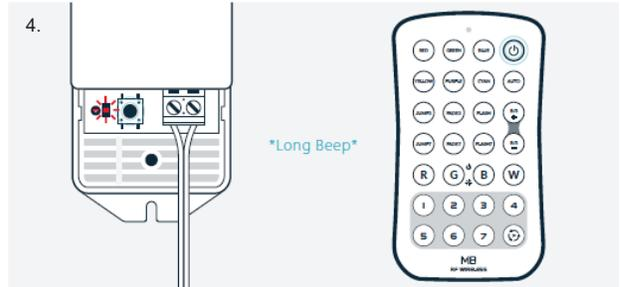
Press the black Sync Button on the receiver once and the the Power Indicator LED will remain static, then quickly press any button on the remote and the Power Indicator LED will flash faster then continue flashing at a slower pace as before. The remote is synced. (To reset the receiver and try again, press and hold the sync button until it beeps twice (about 10 seconds). The receiver is reset)
