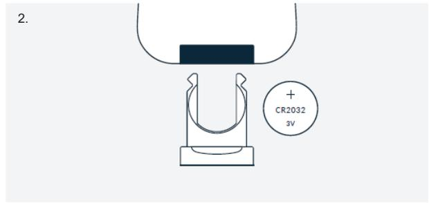
Open the tray on the back of the remote and make sure the battery doesn't have the protective plastic.
