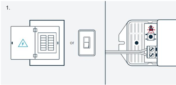
Turn the main breaker for the AC line back on to power your non-dimmable power supply. The red Power Indicator LED on the receiver will start flashing slowly demonstrating that it's getting power. The receiver is located inside the lighting fixture.
