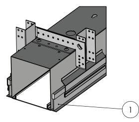
Use support cable to support fixture, by tying through any of the three holes on the top of the yolk.
