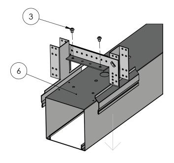
Anywhere along the length of the fixture, slip 2 assembled Retrofit Yolk Assemblies over the top of the fixture. (Note: it will be a snug fit)
