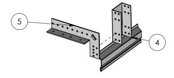
Secure yolk top to each yolk arm by driving 2 self-tapping#8 screws through holes indicated in drawing.
