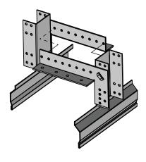
Secure the 2 yolk halves together driving 2 self-tapping#8 screws through holes indicated in drawing above. For a 44 fixture use the last availables for the snuggest fit.
