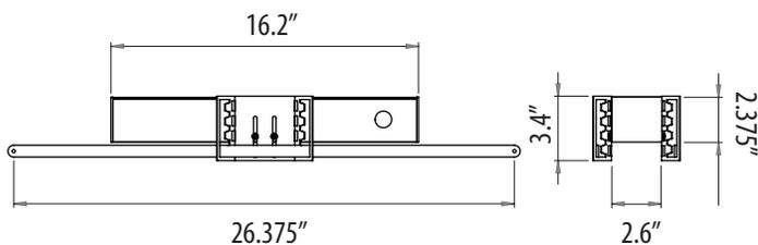
Insert cable ends into grippers. Depress gripper nozzle to release/adjust cable. After final adjustments, leave approximately 1 inch of cable out of exit hole.
