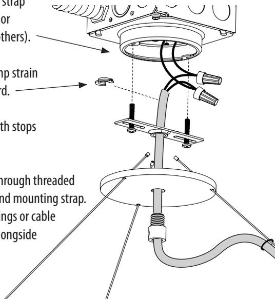
**NOTE:** Maximum canopy to fixture distance: 25 ft. Maximum canopy to driver distance: 100 ft. (with 10 AWG wire).
