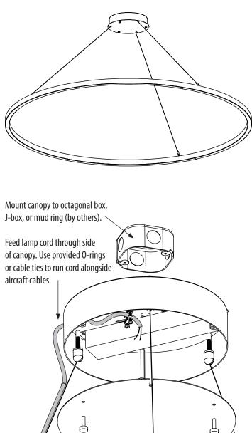
**Direct Only wiring:** Red to 24VDC positive Blue to 24VDC negative
