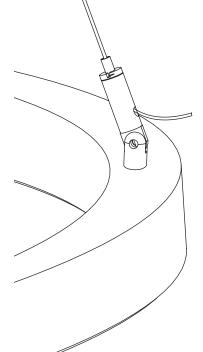
**NOTE**: Maximum canopy to fixture distance: 25 ft. Maximum canopy to driver distance: 100 ft. (with 10 AWG wire).
