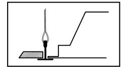
Flange Kit in ceiling opening and wire support each corner to ceiling structure. (at four corners as shown)
