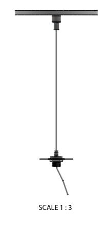
First slip your cable into the CC 1/4-202P all the way to the cable stop
