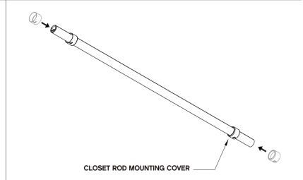
3 INSTALL ONTO CLOSET ROD MOUNTING BASE SUPPORT.
