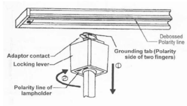
**CAUTION:** Before installing track head, make sure hot contact conductor is on the right position.
