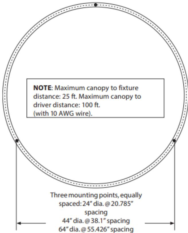
Mount driver housing to octagonal box or mud ring. Wire up drivers to line voltage on primary side.
