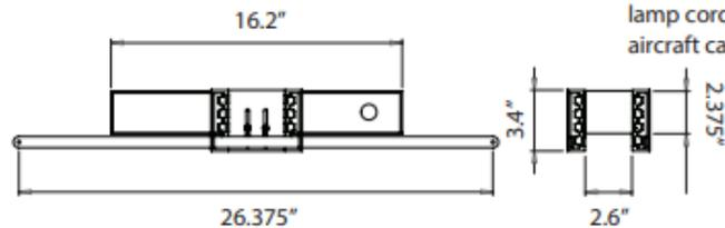
Remote driver includes bar hangers to mount above suspended ceilings. Drivers must remain accessible after installation.
