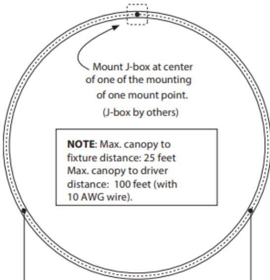
Three mounting points, equally spaced:
