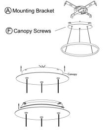
Twist canopy to lock fixture in place. Secure canopy with canopy screws (F).
