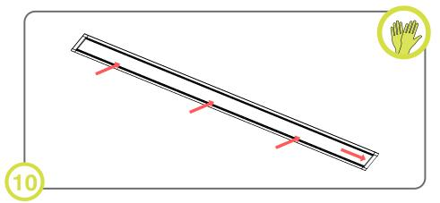
Repeat step 8 on the other side. Starting at one end, press the rest of the lens into the Vesta to complete installation.
