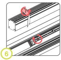
Turn screw to rotate bracket and secure to ceiling until gasket compresses adequately
