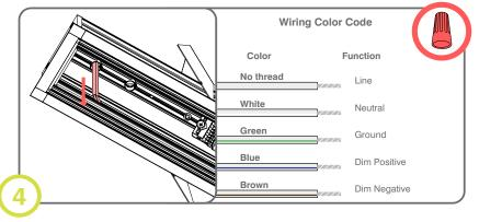
Feed wire through bushings. Make electrical connections.
