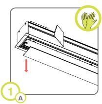
Carefully detach lens starting from the gasket end. DO NOT remove from the side as this may cause cracking.
