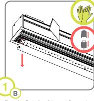
Separate reflector from fixture and disconnect.
