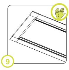
Slide lens until sealed against rubber gasket.
