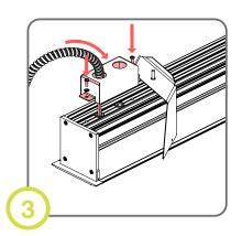
Feed BX cable into termination box and install on Vesta. BX connectors supplied by others.
