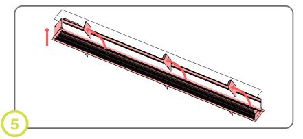
Collapse brackets and slide fixture into ceiling. For uneven surfaces, apply silicone around flange before installing Vesta.
