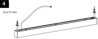
Locks the fix plates on fixture using the PM4 screws
