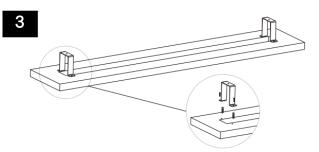
Lockes the brackets on site using the wall anchor and PA4 screws
