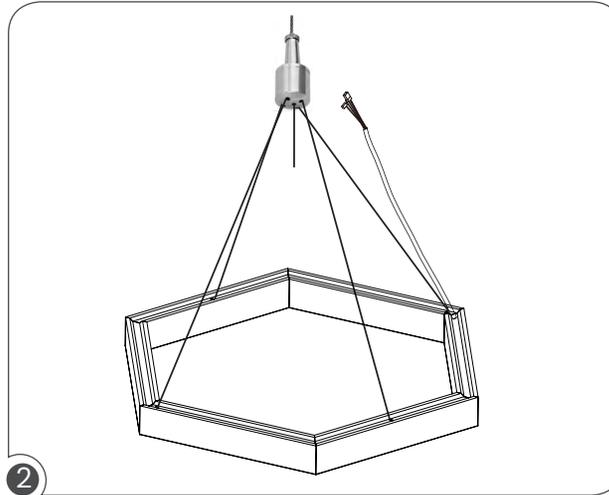
Twist top of the pre-installed gripper to loosen the entrance, insert cables, and lock grippers. Adjust to the desired suspension length.
