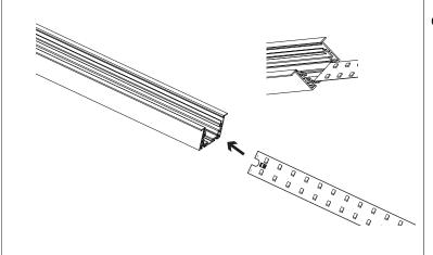
6 INSTALL DIFFUSER ONTO PROFILE
