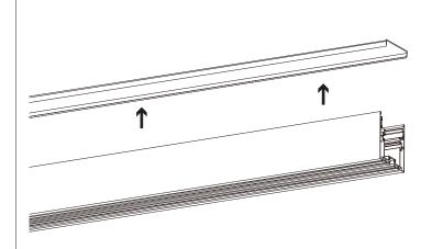
MAKE A SLOT THE SAME SIZE AS THE PROFILE ON THE CEILING TO ACCOMODATE CHANNEL
