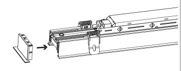
9 CONNECT POWER SUPPLY TO WIRE IN CEILING THEN INSTALL PROFILE INTO SLOT.
