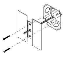
Align the bracket to the gap on the wall plate / canopy kit then mount the bracket using the screws provided. Secure the bracket tightly.
