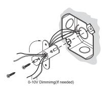
Mount the wall plate / canopy kit to the crossbar using the screws provided
