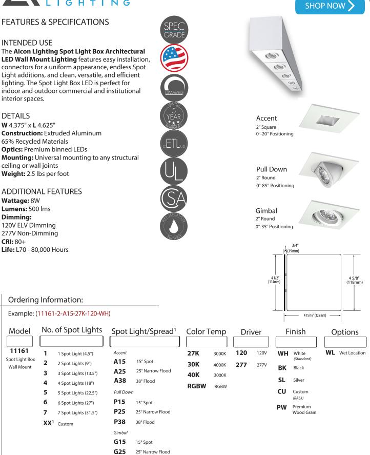
Alcon Lighting **11161 Spot Light Box** Architectural LED Linear Suspension Wall Mount Fixture
