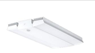
LED High Bay fixture ideal for large indoor spaces, including warehouses, gymnasiums and distribution centers that require mounting heights from 15 to 50 feet. An integrated motion/photo sensor option provides multi-level lighting control. Available in 95, 150, 185 and 225 Watt versions with equivalencies from 200 to 400 Watt metal halide fixtures.
