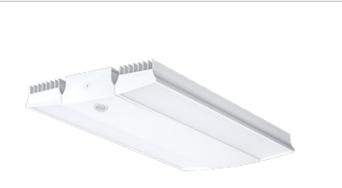
LED High Bay fixture ideal for large indoor spaces, including warehouses, gymnasiums and distribution centers that require mounting heights from 15 to 50 feet. An integrated motion/photo sensor option provides multi-level lighting control. Available in 95, 150, 185 and 225 Watt versions with equivalencies from 200 to 400 Watt metal halide fixtures.
