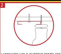
LUMINAIRE HOLE CUTTING TEMPLATE: Two people are required to use the metal template. A rotary tool with a 1/8" bit is required to cut the luminaire hole.
