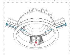
Once flush against the ceiling plane, push the 3 arms back out of the fixture body. Using a standard screwdriver, pull the arms down to securely clamp the fixture to the ceiling panel.
