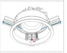
Once flush against the ceiling plane, push the 3 arms back out of the fixture body. Using a standard screwdriver, pull the arms down to securely clamp the fixture to the ceiling panel.
