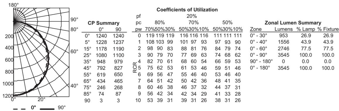
2FSL2 40L LP835, test no. LTL24691P9, tested in accordance to IESNA LM-79
