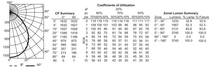
2GTL4 LP835, 4006.7 delivered lumens, test no. LTL22798, tested in accordance to IESNA LM-79.
