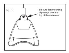
Step 2: Hang the fixture from suspension cables by hooking into each end of light fixture. Install 10-32 flange nuts from the hardware kit onto threaded cable end (Fig. 5) and adjust up or down as necessary until fixture is level (Fig. 6).
