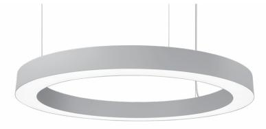
High Performance 4" Aperture Circle (HP-4 C) is a patented, circular LED luminaire. Constructed with an extruded aluminum body and single-piece diffuser, the HP-4 C provides a seamless finish aesthetic. Delivering excellent performance using an advanced optical design and mid-power LEDs to achieve 90% of initial light output at 100,000+ hours.
