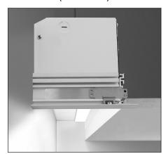
Adds 1-1/4" for Spackle Flange and 1" for T-Bar (includes endcap dimension 1/8") per endcap to the housing length on shop drawings. T-Bar version shown, Spackle Flange available.
