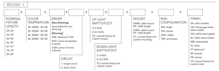
Note: Remote driver ordered separately, refer to supplemental driver details sheet for availability. \* A standard finish requiring a two step coating process, premium will apply.
