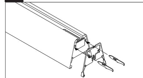
Slide joiner aligner brackets into corresponding slots in fixture cross plate.
