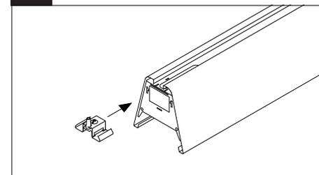
Slide A/C mounting bracket into mounting channel to the mounting position, and tighten locking bracket until screw is tight. **Mounting position can be up to 18" from end.**
