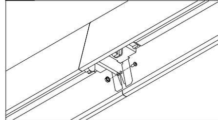
Slide modules together; secure joint from below using supplied nut and screw hardware (requires Phillips driver). **IMPORTANT:** Ledalite recommends tightening fasteners by hand. When joining modules, ensure screw is tightened snug plus an additional 1/4 turn. **LEVEL FIXTURE:** See **A** below. Repeat STEPS 4-7 for each additional fixture in row.
