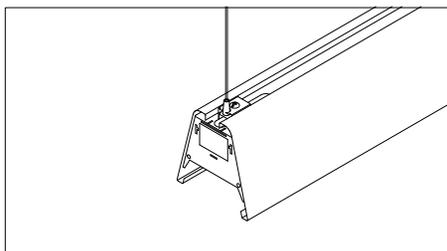
With two people, raise first fixture to ceiling. At each end of fixture, insert aircraft cable through aircraft cable adjuster (located on A/C mounting bracket). The adjuster will automatically grip and hold the cable.
