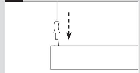
**LEVEL VERTICALLY** (shown above): Support fixture from below and use supplied aircraft cable release tool to make fine height adjustments (see instruction A for details).
