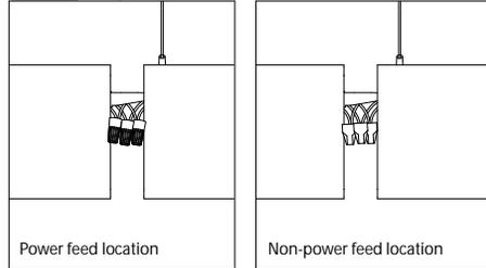
Complete in-run electrical connections. **NON-POWER LOCATIONS** (shown above): Use supplied quick-wire connectors. Tuck wires into wire cavity. **POWER LOCATIONS:** Feed power cord through bushing in bracket. Use wire nuts (supplied by others) to complete connections. Tuck wires into wire cavity.
