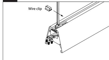
**POWER LOCATIONS:** Attach cable clips at 4" increments between power drop and bushing in power cover. Feed power cord through bushing (shown above). Complete electrical connections using wire nuts (supplied by others). Tuck wires into wire cavity.
