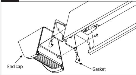
Snap on the gasket to the end of the fixture and attach end caps using supplied #8 screws.
