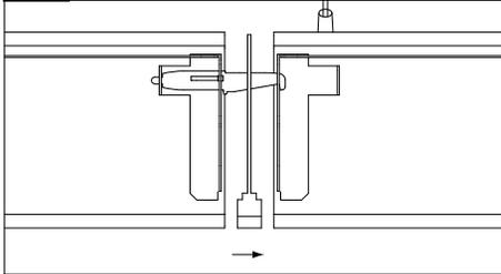
With two people, raise second fixture to ceiling. At end of fixture (opposite joint), insert aircraft cable through adjuster. At joint, rest fixture on in-run joiner bracket. **IMPORTANT:** Do not attempt to join fixtures on floor. Instead, hang one fixture at a time and join modules at ceiling level.
