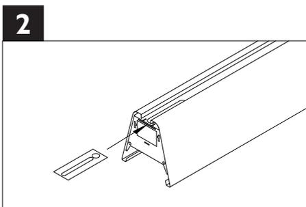
Slide in power cover and install bushing (power location) or plug (non-power location) on both ends. Install one gasket per joint.
