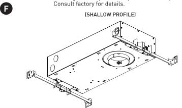
IC HOUSINGS Housing used depends on specified lumen package. Consult factory for details.
