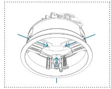
Simply remove the pop-off baffle and depress 3 metal arms into the fixture body. The fixture inserts up and through the cut-out. No housing required in many installations.
