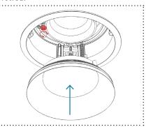
Make desired adjustments to tilt and rotation. Insert baffle up and in to the aperture until it nestles into place.
