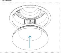
Insert baffle up and in to the aperture until it nestles into place.
