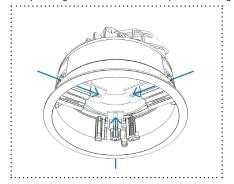
Simply remove the pop-off baffle and depress 3 metal arms into the fixture body. The fixture inserts up and through the cut-out. No housing required in many installations.
