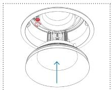
Make desired adjustments to tilt and rotation. Insert baffle up and in to the aperture until it nestles into place.
