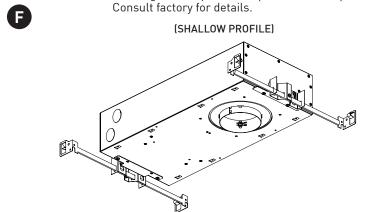
IC HOUSINGS Housing used depends on specified lumen package. Consult factory for details.
