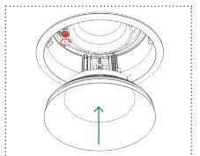
Make desired adjustments to tilt and rotation. Insert baffle up and in to the aperture until it nestles into place.
