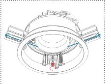
Once flush against the ceiling plane, push the 3 arms back out of the fixture body. Using a standard screwdriver, pull the arms down to securely clamp the fixture to the ceiling panel.
