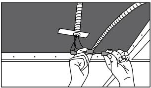
Step 2: Mount knockout plate to flex conduit. Connect pigtail to conduit wires.
