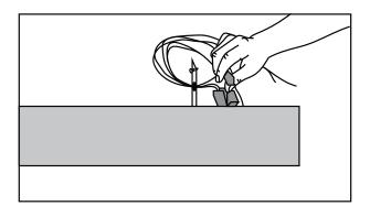
Step 1: Shut off power. Remove ceiling tile from desired light fixture location. Remove knockout plate. Remove pigtail.
