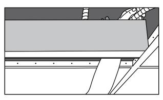
Step 3: Lay luminaire in grid at desired position. Secure fixture to structure above using structural wire (by others) via holes in the end plates.
