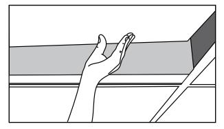
Step 5: Cut tile to fit beside luminaire and install on both sides of the luminaire.
