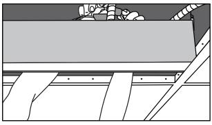
Step 4: Connect pigtail disconnects to luminaire disconnects. Insert wires into housing. Insert knockout plate and fasten using screw provided.
