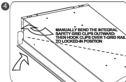
Bend the safety grid clips 90° with hand, then secure the clips over T-grid rail to lock-in position. Check to make sure the fixture is firmly fixed on the T-bar grid.
