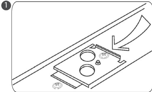
Look for the access plate on the back to access the wires.
