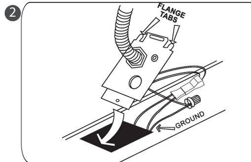
Punch a knockout and make proper wiring connections including a ground wire.
