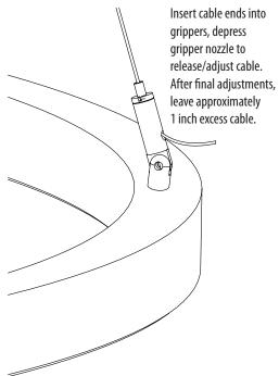
hub top cap; insert cable through top cap and into gripper nozzle.
