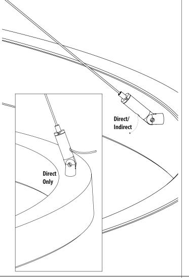
**NOTE**: Maximum canopy to fixture distance: 25 ft. Maximum canopy to driver distance: 100 ft. (with 10 AWG wire).
