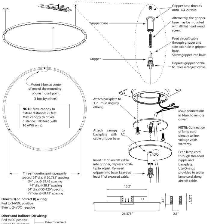
Blue to DC negative \_\_\_\_\_ Driver 1-Indirect Red/White to DC positive Blue/White to DC \_\_\_\_\_ Driver 2-Direct negative
