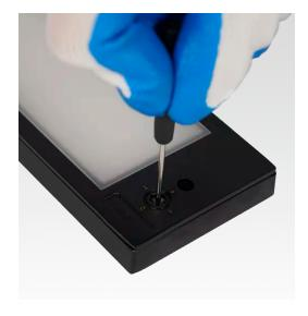
You can adjust both power and CCT on this fixture. Use the provided flat screwdriver to turn the power adjustment screw clockwise or counterclockwise until you reach the desired brightness.
