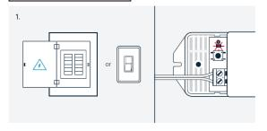
Turn the main breaker for the AC line back on to power your nondimmable power supply. The red Power Indicator LED on the receiver will start flashing slowly demonstrating that it's getting power.
