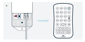
Press the black Sync Button on the receiver once and the the Power Indicator LED will remain static, then quickly press any button on the remote and the Power Indicator LED will flash faster then continue flashing at a slower pace as before. The remote is synced. (To reset the receiver and try again, press and hold the sync button until it beeps twice (about 10 seconds). The receiver is reset)
