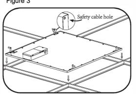
Insert luminaire into T-bar ceiling grid. Secure safety cable to connection hole as needed to meet local seismic requirements. Safety cable and method of attachment to the building provided by contractor according to local
