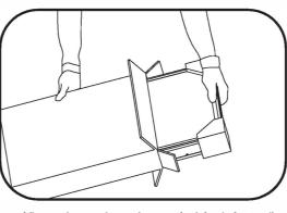
Carefully unpack unit and properly inspect for defects before installing. Wear work gloves to prevent dirt and oil from being transferred to the luminaire. If cleaning is needed, use gloves and a dry cottoncloth. It is not recommended to use hazardous chemicals.
