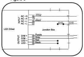
Follow wire connection instructions. When using the 0-10V dimming controller Run wires from controller through a different knockout than the AC input wire. Don't forget to return the electrical enclosure cover and tighten the screws.
