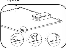
Lift up four mounting clips on the sides of the luminaire. You can do it by hand(Do wear work gloves) or use pliers
