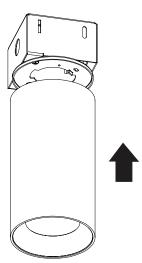
4 Turn clockwise until secure. Note: For wet location, apply caulking between ceiling and cylinder.
