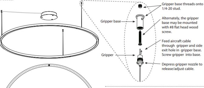
**NOTE**: Maximum canopy to fixture distance: 25 ft. Maximum canopy to driver distance: 100 ft. (with 10 AWG wire).
