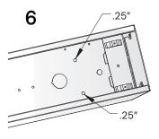
Mount fixture to surface by installing screws through .25" holes (or keyways if applicable) located on back of fixture.
