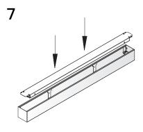
Wire fixture according to all national, state and local codes. Re-install LED assembly and test fixture.
