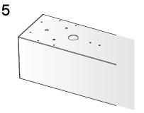
7/8" knockout is located on the back of the fixture to allow for wiring. Bring wiring through.
