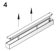
Remove LED assembly (it will hang from tethers) and set aside.
