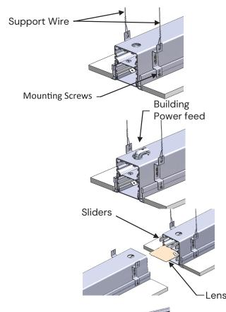
Fasten extended reflector tabs to joining fixture. Break tab at end of run.
